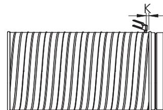
2.1. For saddling a saddle (NPS-T, NPSK-T or NPSV-T) is recommended, as this will enable connection without cutting apart a duct. Place the saddle on the duct and draw the saddle contour on the duct surface. Cut a hole into the duct about 10 mm smaller than the contour. Start cutting from the centre hole of the area to be cut. Apply a sealing compound on hole edges before attaching the saddle. Place the saddle in the correct position and attach.
